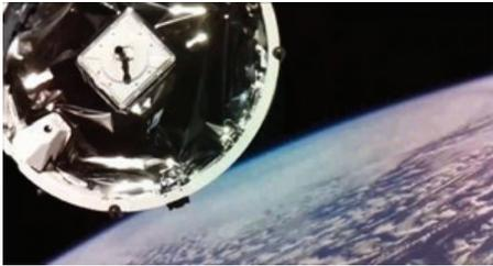
rocket included a previously undisclosed kick stage designed to increase orbital options for small satellites. The kick stage is equipped with its own avionics, power and communications systems, and Rocket Lab plans to offer it as an option for future flights. "With the new kick stage, Rocket Lab can execute multiple burns to place numerous payloads into different orbits," the company said. To minimize space junk, the kick stage is designed to de-orbit after it finishes its
